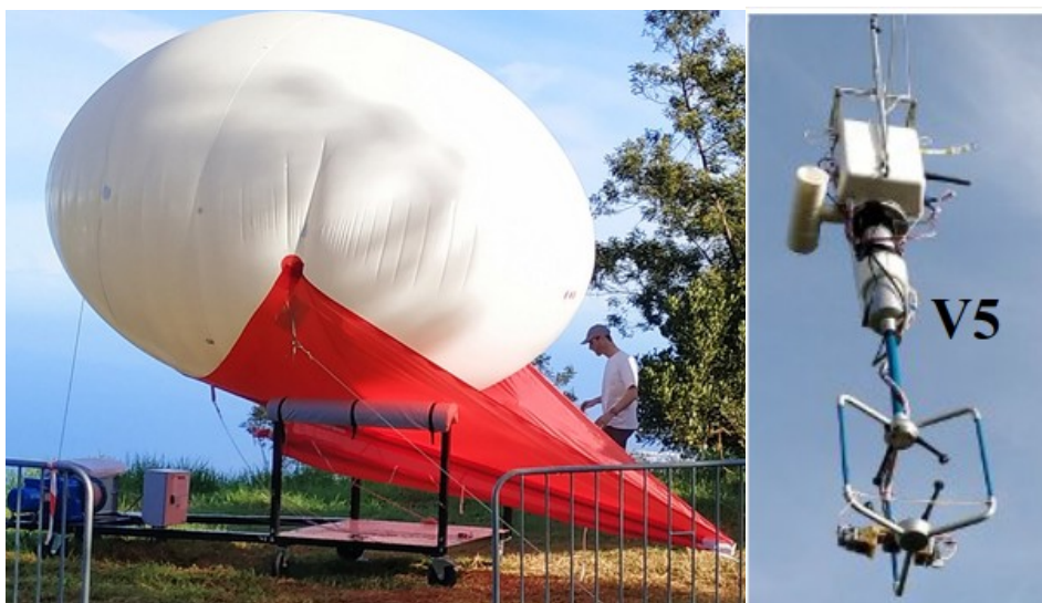
Figure 9: The Skyhook Helikite 16m 3 tethered balloon and the turbulent probe
